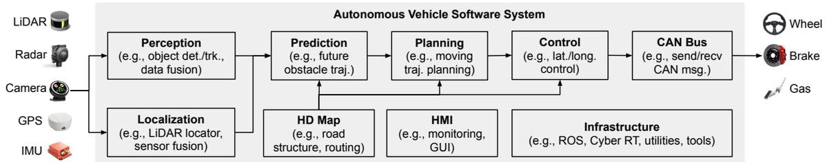
**Figure 1: State-of-the-art Autonomous Vehicle (AV) software system architecture from most popular AV development classes such as Udacity Self-Driving Car Engineer classes [20] and real-world AV systems such as Baidu Apollo [4] and Autoware [3].**
